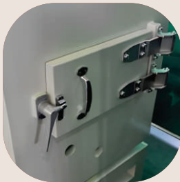
Added Door & Utility Pipe
